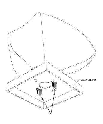
5. The tension of the basin tilt mechanism can be adjusted by tightening or loosening the spring tension bolts (1). WARNING: DO NOT ADJUST BY MORE THAN 2 FULL TURNS IN EITHER DIRECTION.
